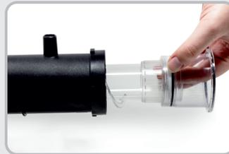
The quartz sleeve can be coated in limescale build up in hard water areas. This should be carefully removed from the quartz sleeve and cleaned with a soft cloth.
