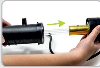
To access quartz sleeve loosen it up by inserting a flathead screwdriver between the quartz sleeve and quartz sleeve housing (see reference image below). Gently pull it out to remove it.
